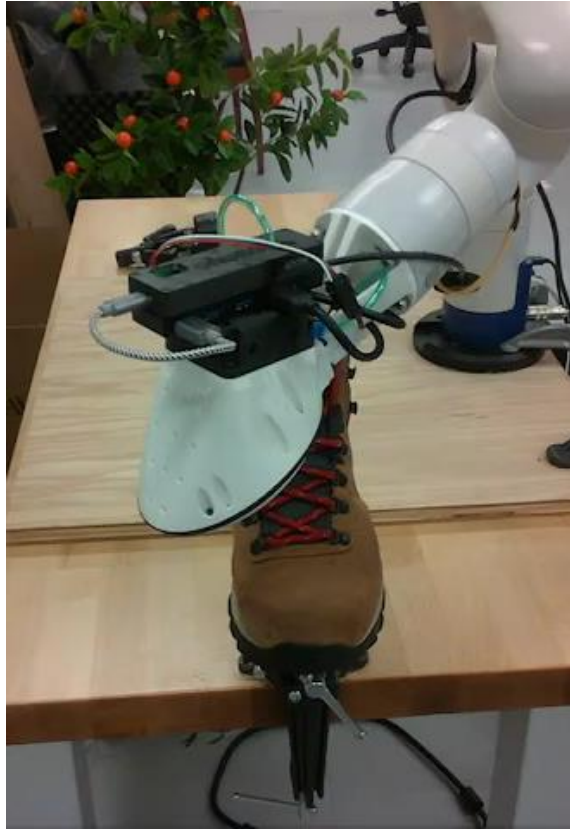
Soft bubble sensor, Alspach et al., RoboSoft, 2019
